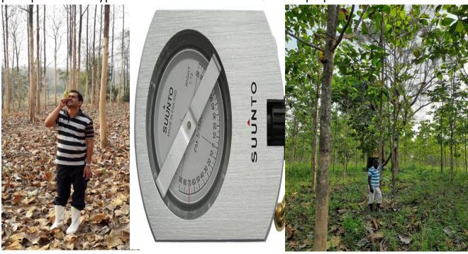
Figure 3. Total Tree height was measured by hypsometer and a pole, used instrument of sununto meter is shown in above
